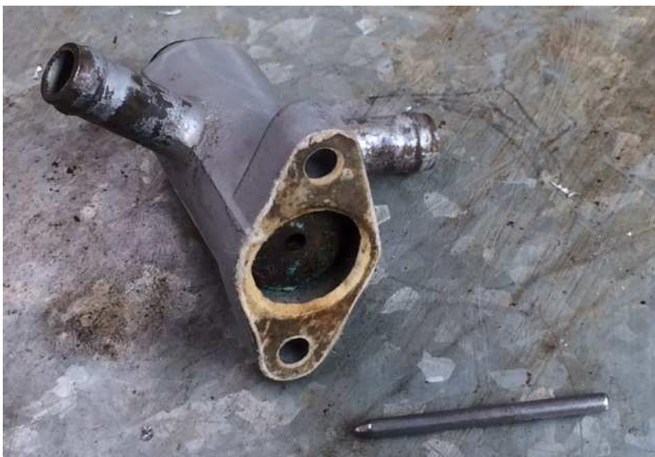
This shows the heating assembly and control pin after removal from the air slide assembly.
