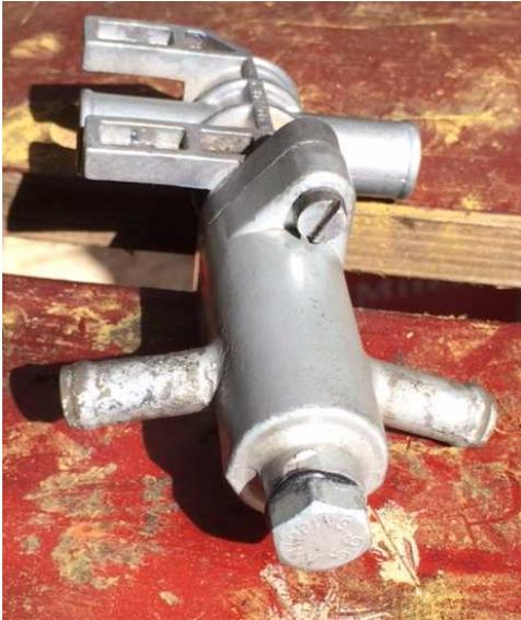
Whilst a fair bit of information exists about repair and adjustment of the Warm Up Regulator fitted to E21 BMW's with the Bosch K Jetronic fuel injection system, I found very little information on one of the other key components of the K Jetronic system, the additional air slide valve.
