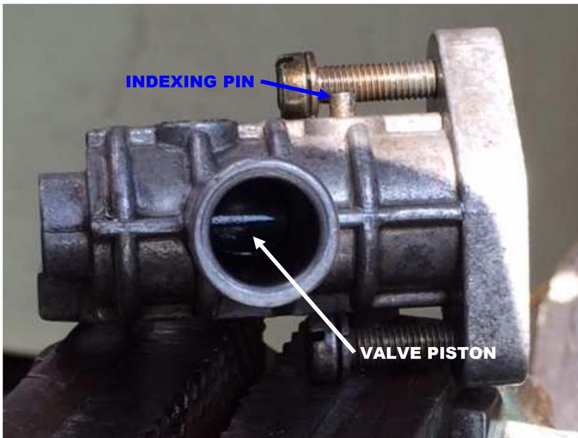
This is the business end of the valve—the air slide valve. Note that in this photo the valve is jammed fully closed, it was initially jammed in the fully open position and closed as the result of me spraying it with copious amounts of Inox (like WD-40) and tapping the flat area of the valve piston in an attempt to free it up.
