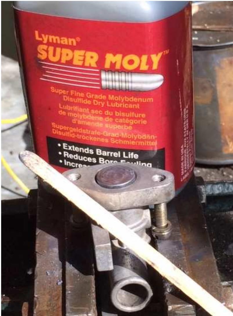
Lubricate the piston bore by pushing the piston to the bottom of its stroke with a piece of dowel, then introduce a small amount of molybdenum disulphide powder and work the piston up and down in the bore to evenly distribute the powder.
