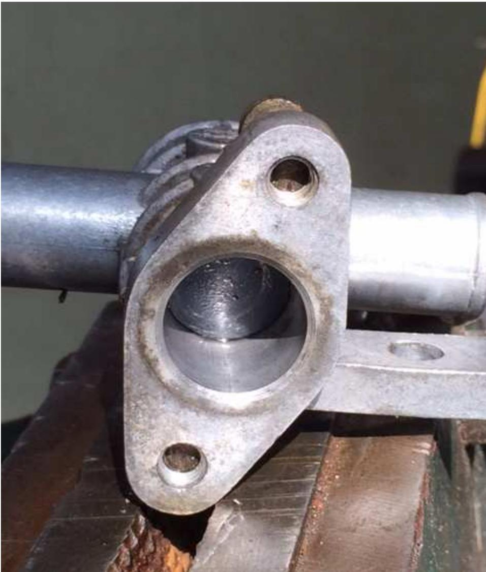
You can see the air slide piston here, stuck at the bottom of its bore.
