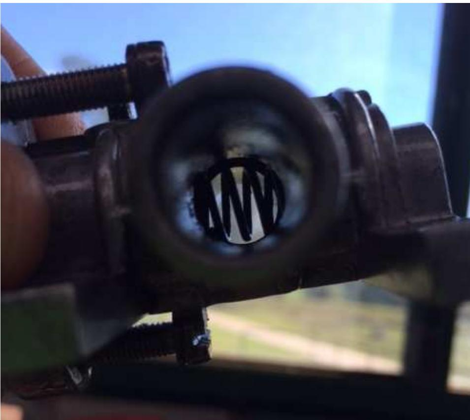
Once the piston has been fully freed up, the spring should force the valve wide open.
